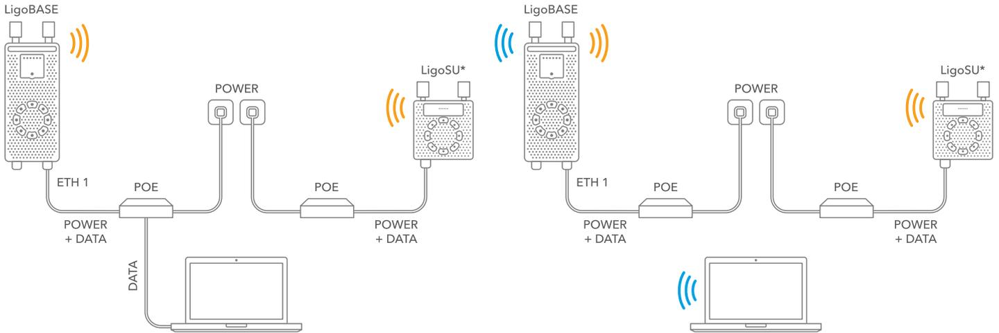
\*Multiple LigoSU units can be connected to the LigoBASE
