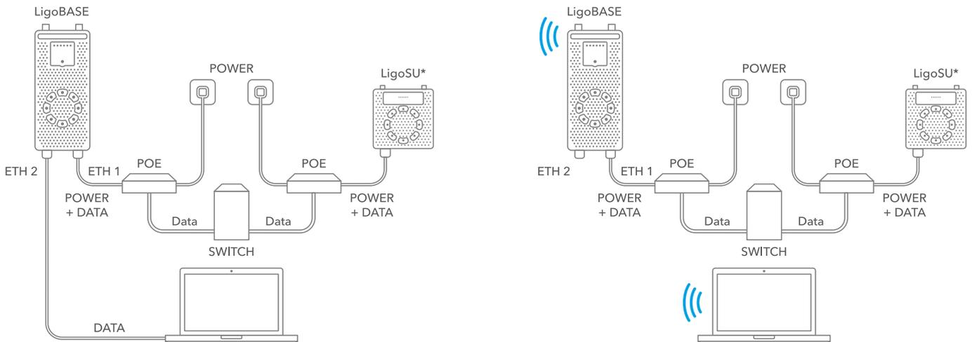
\*Multiple LigoSU units can be connected to the LigoBASE
